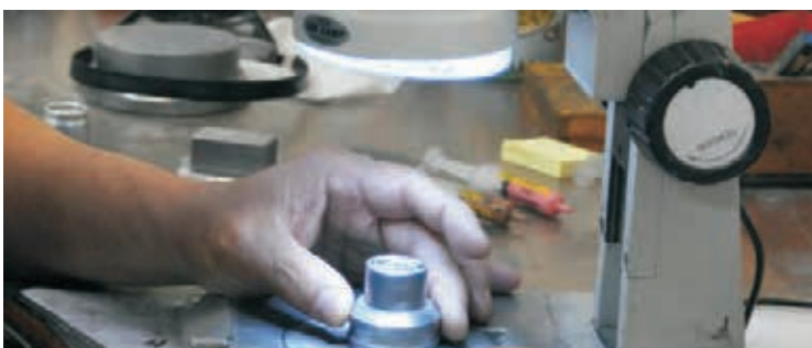
Hand engraving fine detail into a master die.
